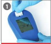
Pull the backside of the cuvette holder slightly towards you and lift up
