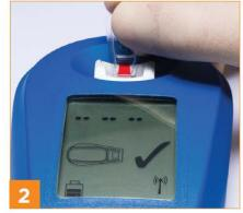
Insert the filled cuvette and press down gently
